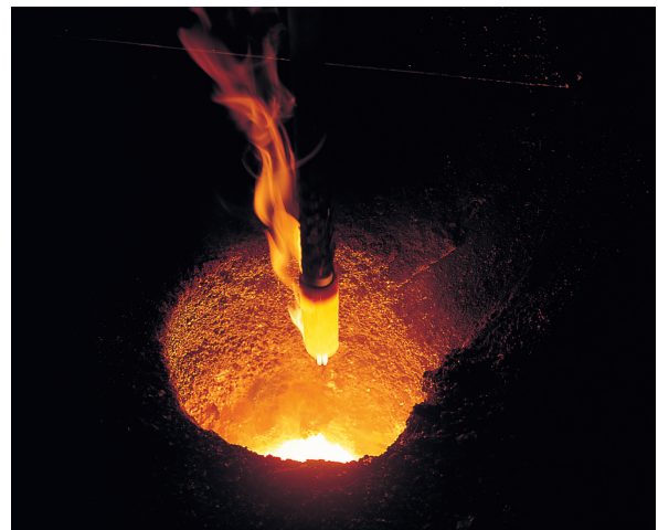
The Celox® sensor after an oxygen measurement
