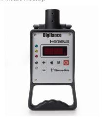
The instrument has been developed to allow measurements with the C-V-Therm sensors as well as Positherm®-Al sensors, giving the flexibility and autonomy for selecting the correct type of probe.
