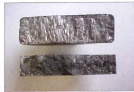
FIG. 9 : Example of a white (top) and grey (bottom) solidified hot metal sample
