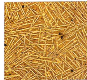
FIG. 10 : Microstructure of a hot metal sample taken in the desulphurisation station with a pocket sampler. The presence of needles and very few graphite inclusions indicates a good white solidified sample structure.
