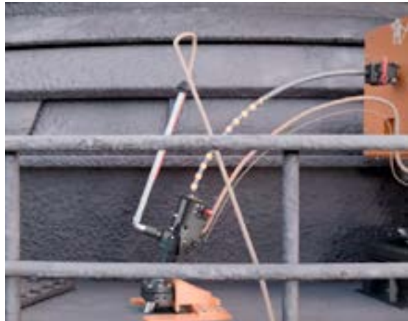
Blowing lance on the horizontal panel
