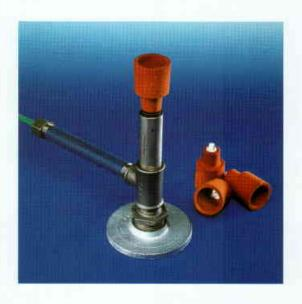
This is Heraeus Electro-Nite's simplest option for rapid carbon determination. Fitted with a high grade type S (Pt 10% Rh/Pt) or type R (Pt 13% Rh/Pt) thermocouple protected by a quartz tube, the Econ-O-Carb\* accurately determines carbon content through thermal analysis.
