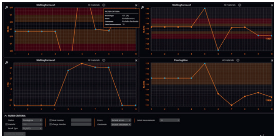
Trending window to trend a result type for the selected station and material. The trend will show the ranges of the different materials measured in that station.
