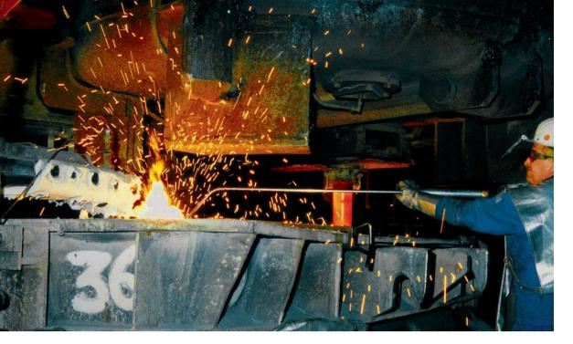
Bath temperature measurement in the tundish
