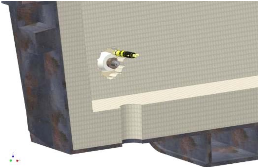
Figure 36 Use a pneumatic hammer to pack the mouldable refractory around the block, filling all gaps.
