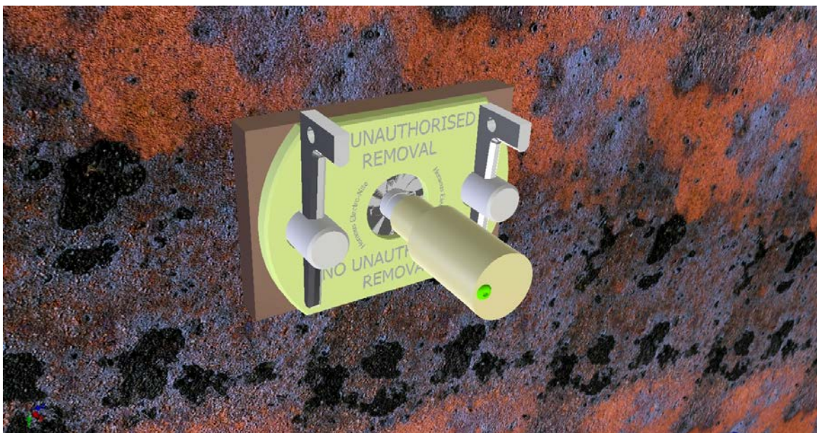
Figure 46 A green light means that the tundish can now be lined.
