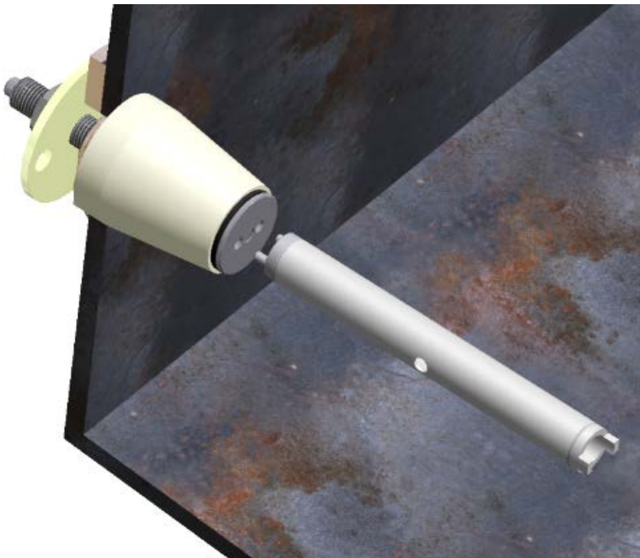
Figure 18 Or you can use the adjustment tool to open and close the embedding tool from the inside of the tundish.
