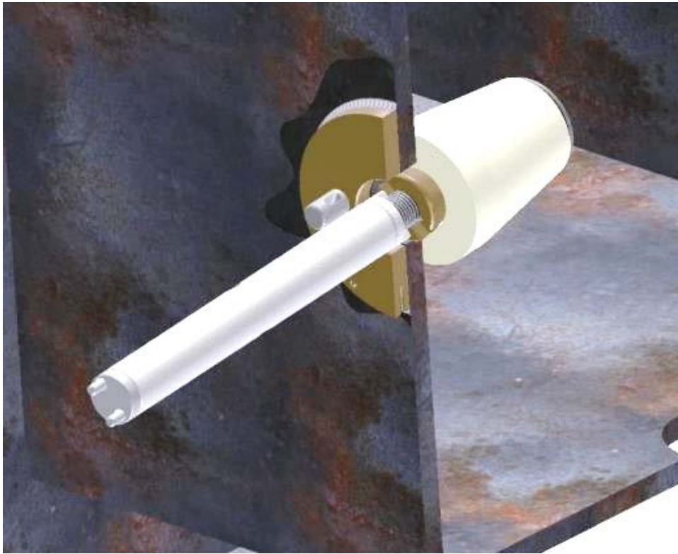
Figure 17 You can use the adjustment tool to comfortably open and close the embedding tool from the outside of the tundish
