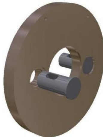
Figure 11 Before welding, consider the best position for the wedges and weld the posts in the appropriate positions.
