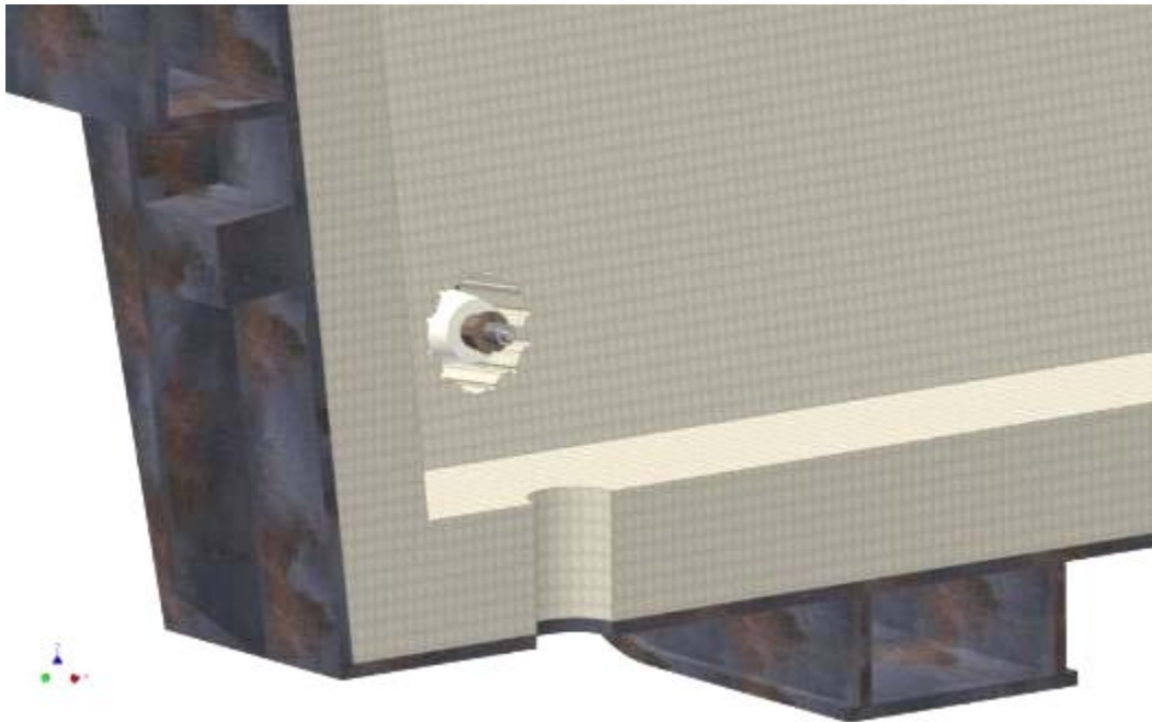
Figure 35 Apply the mouldable refractory once the block is in place.
