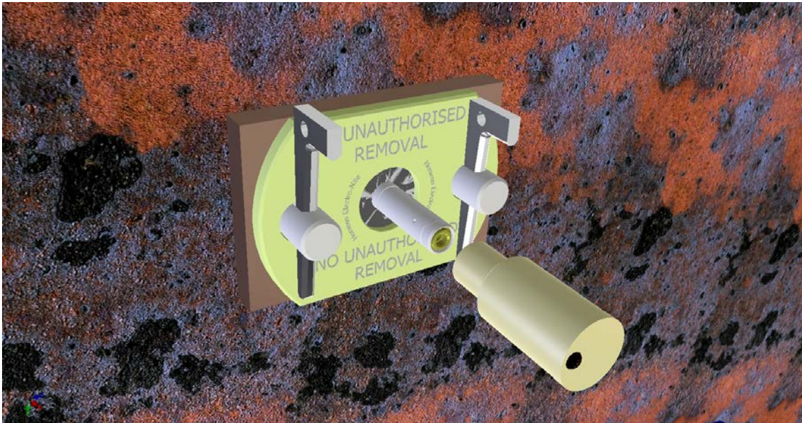
Figure 45 Push the sensor checker onto the sensor
