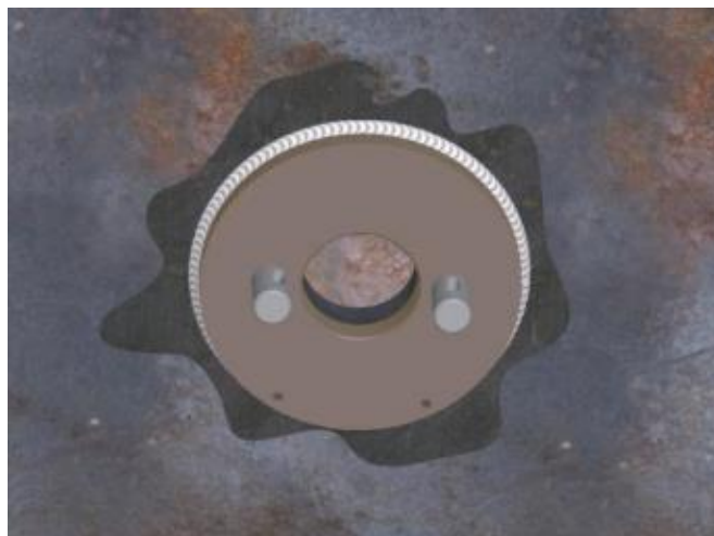
Figure 12 Tack weld the plate against the surface you have ground down, making sure the centre of the plate lines up with the hole. Weld the plate to the tundish (one complete weld plus at least two more complete welds on top of the first one).
