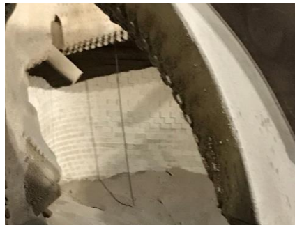
Figure 5. Optical cored wire feeding into the EAF.
