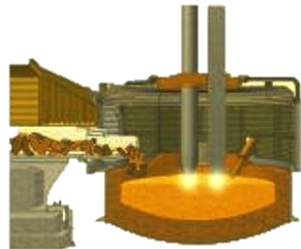
Figure 2. Left, view of the EAF, lintel and Consteel conveyor at NSHC. Right, section view a Consteel EAF. 3
