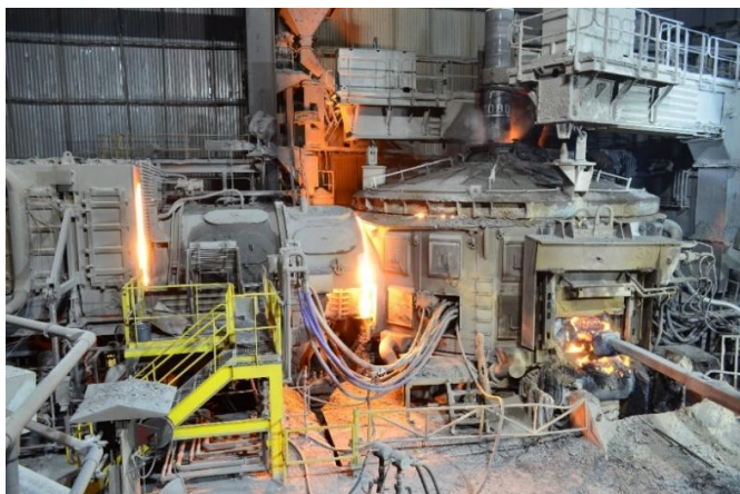
Figure 2. Left, view of the EAF, lintel and Consteel conveyor at NSHC. Right, section view a Consteel EAF. 3
