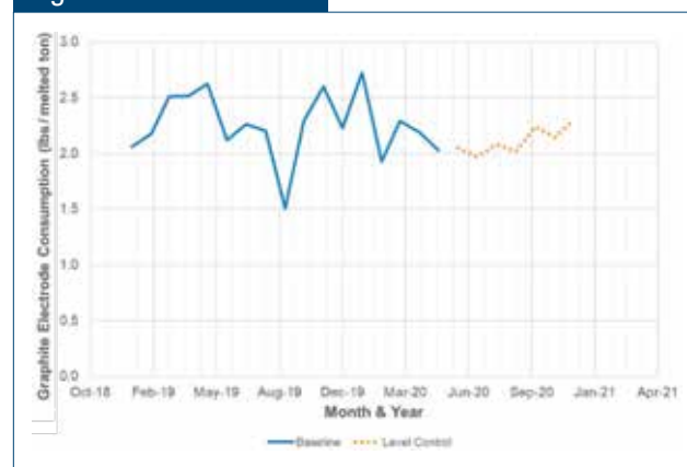
Plot of monthly electrode consumption at the Consteel EAF during the baseline analysis period (blue, solid line) and after implementing level control (orange, dotted line). NOTE: instances of electrode breaks were removed so as not to contaminate the analysis.
