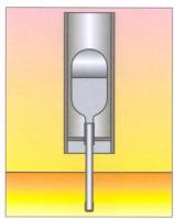
Vacuum samplers are used for sampling from the mould of the continuous caster. Stream samplers are used for sampling from any open stream of liquid metal.
