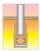
This steel sampler is available in a re-usable tube configuration. The re-usable cardboard tube from a previous temperature measurement can be fixed to the onsert.
