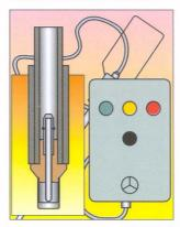
TOS system uses argon flushing before sampling. When using the special pneumatic switch box, the sampling procedure is completely automated.
