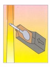
Stream sampling is a safe way to take samples from any open stream of liquid metal.
