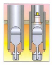
Samp-O-Line® offers standard and customised samplers for all types of steel whenever a homogeneous and representative sample from molten steel is needed. Non-splash samplers are available for improved safety and accuracy. Sufficient immersion depth is required for proper functioning. Capping configuration can be adapted to suit low steel temperatures. As deoxidant e.g. Al, Zr or Ti are available for unkilled steel conditions.
