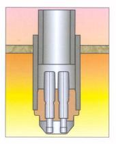
The Double Sampler offers the steel plants the possibility to speed up time for analysis.
