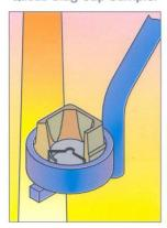
An alternative for the slag immersion sampler is the use of the slag cup sampler, that can be placed in a holder and held in the slag stream when de-slagging the EAF and the AOD.
