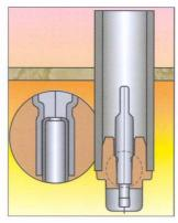
The removal of a sampler pin can in certain circumstances be problematic. The Pin Break Off sampler offers the customer a sample that allows an easy removal of the pin: at high carbon grades, the pin drops off automatically, for low carbon grades, the pin drops off easily by a small hit on the pin.
