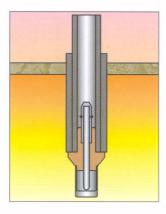
Total Oxygen Sampling offers superb pin sample quality and quick preparation for combustion analysis. TOS is free from contamination, thus being a finger print of the steel cleanliness. Best results are obtained in combination with the special pneumatic lance system in as well RH, ladle, tundish and moulds.
