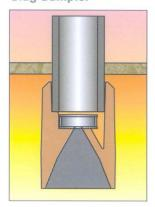
completely new product line is yet available to sample the slag on top of the ladle or converter surface. It provides a slag sample that can immediately be analysed by the XRF without any preparation. The slag sample is obtained after immersion of the slag sampler in the ladle or converter.
