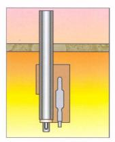
Asingle immersion with the Piggy Back Steel gives both temperature and sample saving time and handling. The Piggy Back Steel is compatible with our standard hardware. Automatic immersion systems take full profit from this combination. As with traditional sampling a wide choice of sample shapes, deoxidant types and tube configurations are available.
