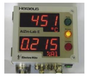
AlZin-Lab E may be connected to a dedicated PC or server PC via a serial Com port or via Ethernet (TCP/IP). Optionally Profibus and Modebus can be offered. The sent data strings may be used for in-plant logistics. The optional AlZinlog PCsoftware makes it comfortable to compute the measured data, and further process it in various Windows programs.
